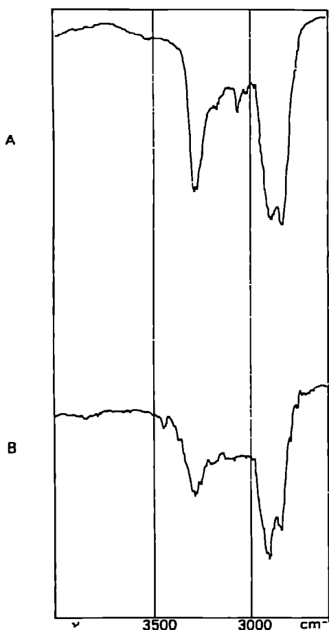
Fig. 1. Part of the IR spectra of the \text{C}_9\text{C}_6 monoamide at 298 K (A) and 323 K (B).
